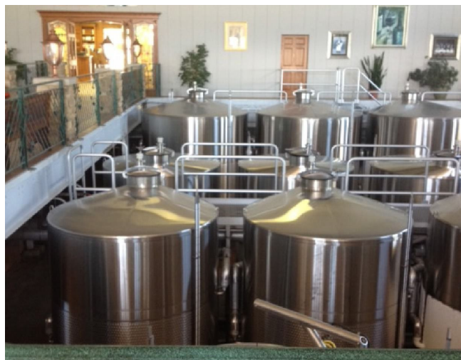
3-Stainless-steel vats with fermenting fruit-of-the-vine. Old-style wooden vats are being replaced here and in Europe by these implements, which allow for more precise control during the wine-making process.
